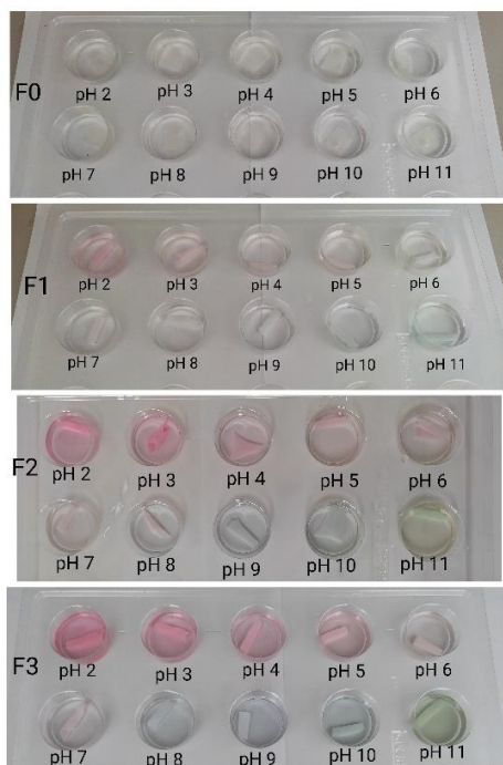
Figure 3. pH Sensitivity of Indicator Films. F0 = without-extract film, F1 = film with 5% of extract, F2 = film with 10% of extract, F3 = film with 15% of extract.
